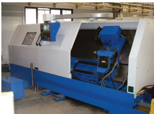
AJSBHD 300-1500 showing powered tailstock
